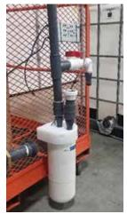
University to design, fabricate and test an integrated water treatment system incorporating advanced ultraviolet light emitting diode (UV LED) disinfection and filtration technologies. The integrated device will target higher flow rates and more challenging water qualities than currently available commercial systems.
