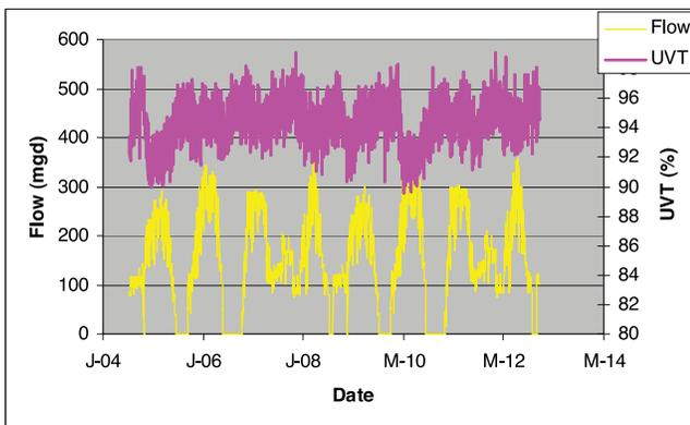
**Figure 5. Flow and UV Data Input into UVCAT**
