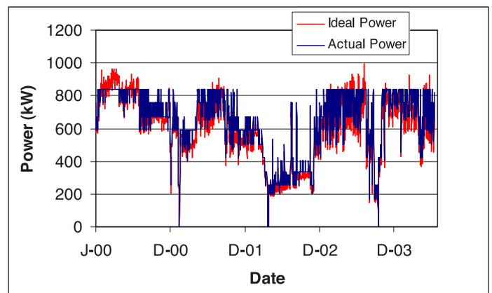
**Figure 7. Power Consumption Predicted by UVCAT**
